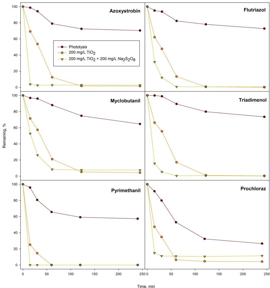
**Figure 1.** Evolution of fungicide residues with the time using  $200 \text{ mg L}^{-1}$  of  $\text{TiO}_2$  P-25 alone or in tandem with  $200 \text{ mg L}^{-1}$  of  $\text{Na}_2\text{S}_2\text{O}_8$  under sunlight. Photolysis curves represent solar degradation in absence of catalyst.
